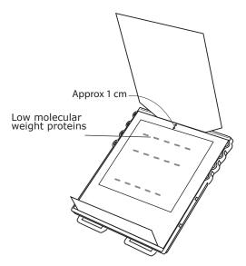
Figure 5. Blot placement
