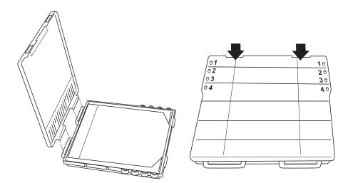
Figure 9. Closing the Immobilon® GO Device
